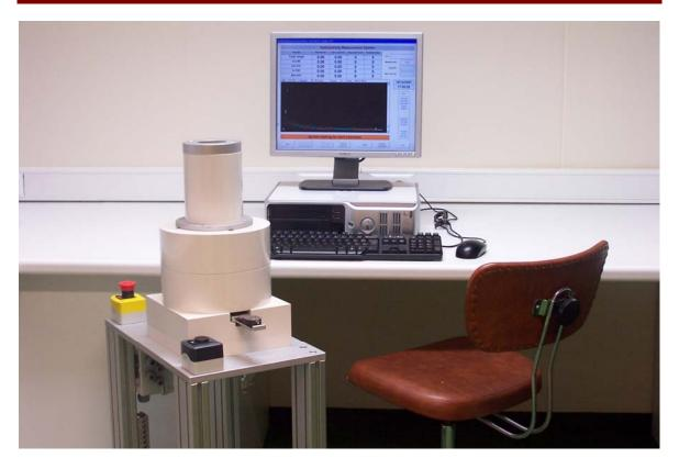
The Radioactivity Measurement System (RMS) is an industrial monitoring tool developed to check cast samples for radioactive contaminants emitting gamma radiation with an energy between 50 keV and 2 MeV.
